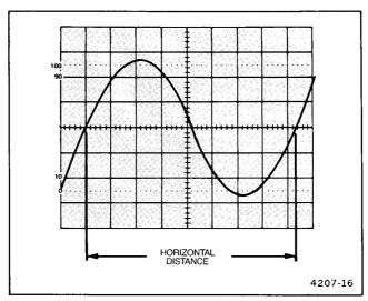
Figure 3-5. Measuring time duration.
