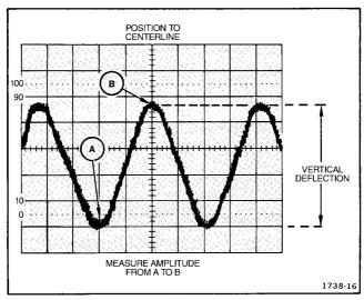
Figure 3-1. Measuring peak-to-peak voltage of a waveform.
