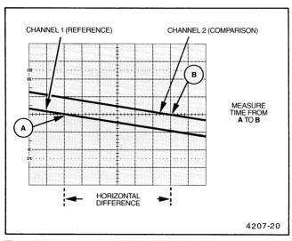
Figure 3-9. High-resolution phase difference.
