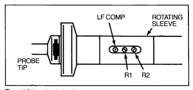
Figure 4-2. Locating the low-frequency compensation adjustment.
