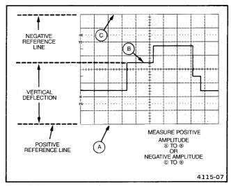
Figure 3-2. Instantaneous voltage measurement.
