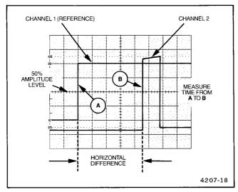
**Figure 3-7.** Time difference between pulses on time-related signals.
