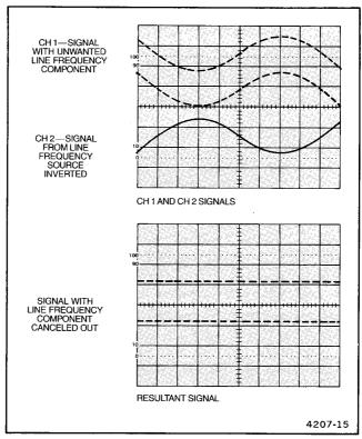
Figure 3-3. Common-mode rejection.
