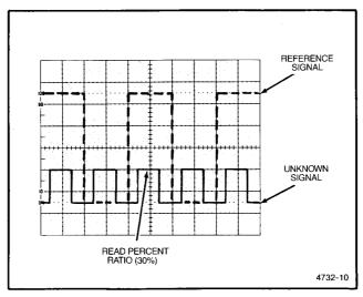
Figure 3-4. Determining voltage ratio.
