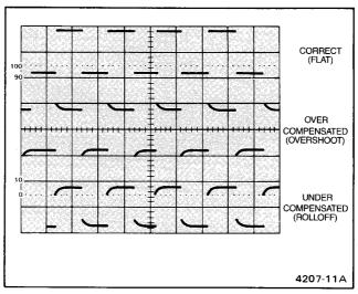
Figure 4-1. Probe compensation.
