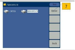
8. Select the downloaded firmware file by rotating the general purpose knob, and then push the Execute bezel button.
